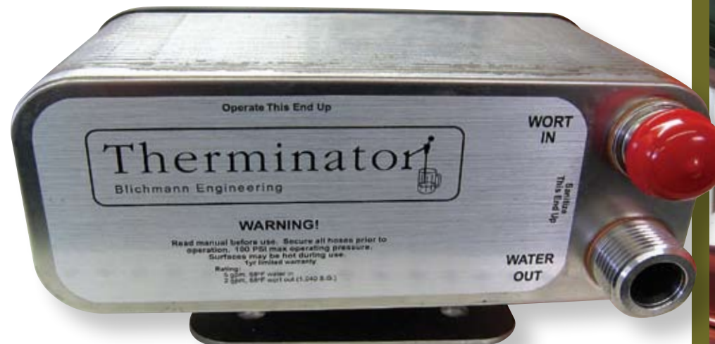
A home-sized version of a plate chiller. Wort goes in one side and comes out the other. There is a separate channel for cool water to flow the opposite direction. The water and wort do not mix.
