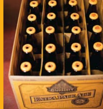
Holes drilled in the caps where dissolved-oxygen samples have been taken.
